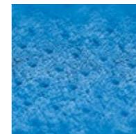
Damaged fibres as a result of prolonged washing from normal washing machines.
